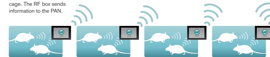
PAN is connected to the computer. It receives signal from the RF box that's attached to each cage. The pan can handle up to 127 RF boxes.
