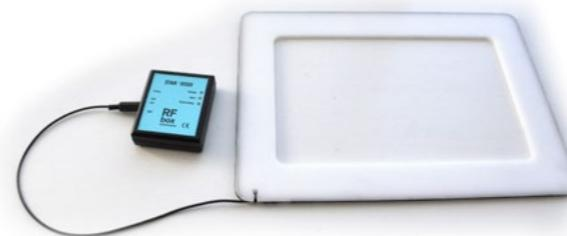
Each cage has an antenna and an RF box. Each receiver can handle up to 10 subjects in each cage. The RF box sends information to the PAN.
